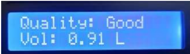
Fig. 6. LCD display showing that water quality is "Good".
